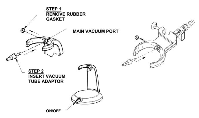
b) Assembly vacuum trap for accepting waste solution between vacuum pump and pedestal or cradle ring stand.
