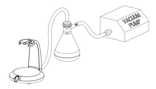
c) Attach feed tube to adaptor and place open end into vessel containing sanitizing agent.
